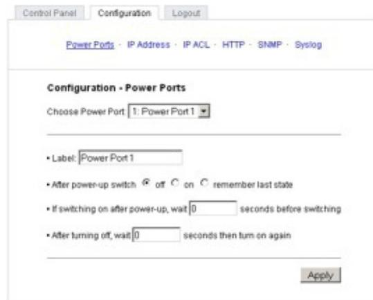
Abb. 5: Configuration – Power Ports
